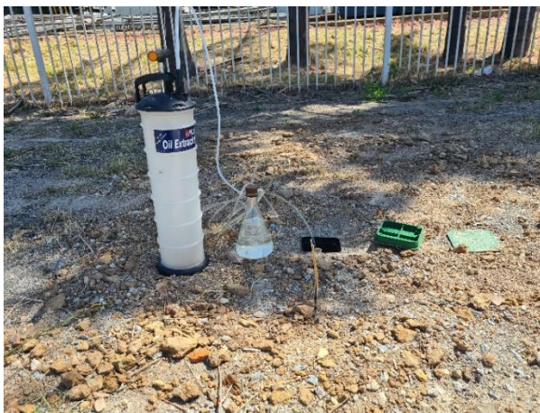
(c) Equipment used to extract water samples from underneath the leaky wells
